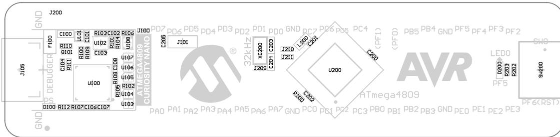
Figure 7-3. ATmega4809 Curiosity Nano Assembly Drawing Bottom
