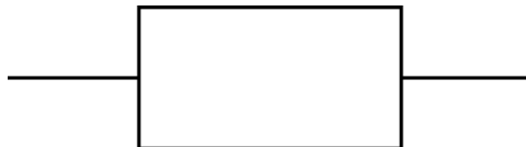
Figur 1: Krettsymbol for motstand
